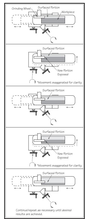
Figure 43. Grinding process illustrated.
